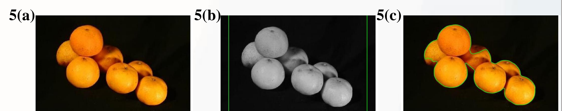
Fig 5. Resolution: 319 \times 383 . Set \Delta t = 2 , \mu = 0.24/\Delta t , binary step c_0 = 2 , \lambda = 3 , \alpha = -3 . (a) original image. (b) proper initial LSF. (c) Set tolerance = 5, after 700 iterations.
